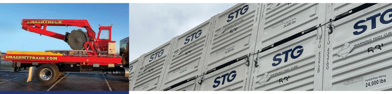
"Smash My Trash" Program: In 2023, STG Logistics introduced the Smash My Trash program. Through the program, a third-party vendor utilizes a mobile dumpster compactor that compresses and compacts waste at STG warehouse facilities. The process makes waste management more efficient and reduces the number of truckloads to dispose of that waste, further reducing GHG emissions. The Smash My Trash program resulted in a 33% decrease in waste management costs at our Compton, California facility in 2023.
